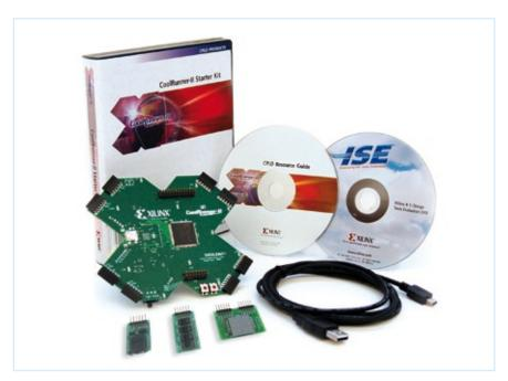
Unlike traditional CPLD starter kit having the peripherals built-in on the starter kit, Xilinx has taken a whole new approach to make it modular so that the designers can easily build and test different peripherals.
